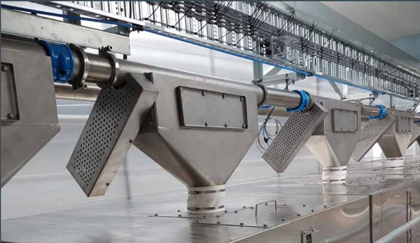
Floveyor's trademark versatility provides a new process line technology solution for multi-outlet material distribution and transfer.
