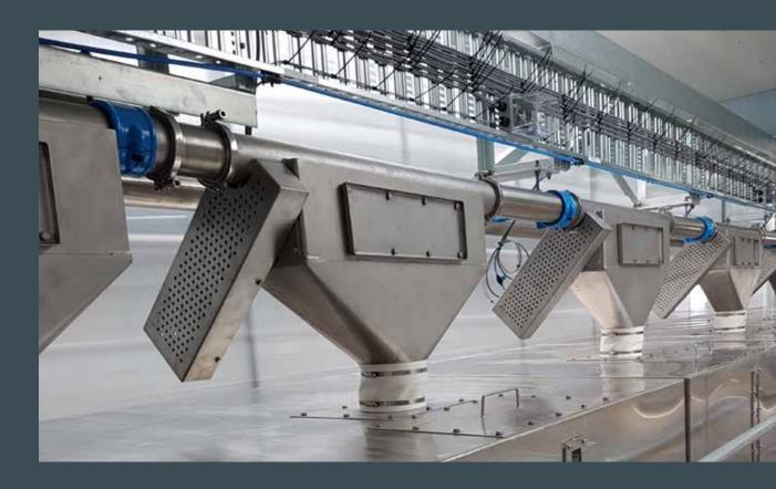
Floveyor's trademark versatility provides a new process line technology solution for multi-outlet material distribution and transfer. Designed exclusively for better powder handling of free-flowing, dry, low-friction powders and granules. The Floveyor Tubular Drag Conveyor is perfect for pet food, animal nutrition, and food and beverage applications.
